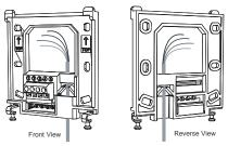
Refer to the diagrams above. Feed the stripped end of the RJ10 cable through the cable guide (see reverse view). Pull through a sufficient working length of cable.
